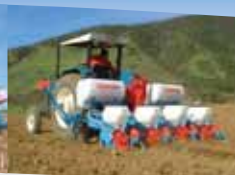
Multi-purpose pneumatic planter with NC shoes
